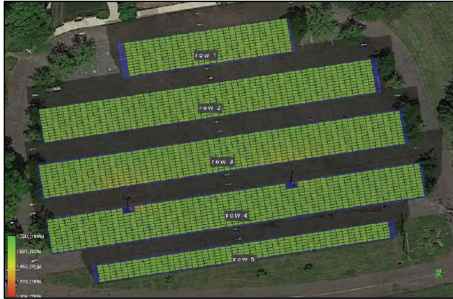
Figure 2 – Design visualization of the Germonds Park parking lot depicting five rows of parking lot solar canopies in the initial construction phase
